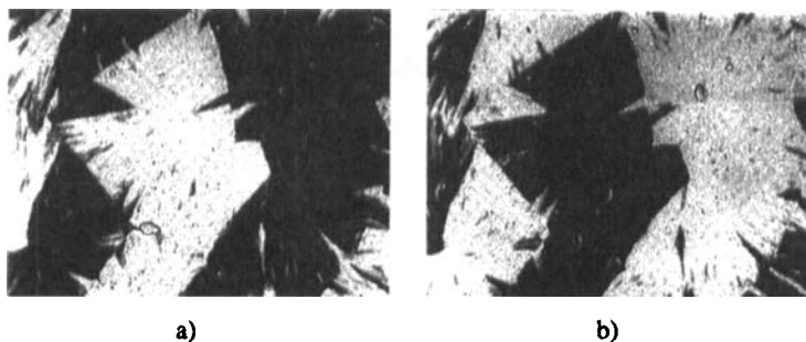
FIGURE 3 Domains of the solid state of compound 9 observed by rotating the analyzer; a) 10° clockwise and b) 10° anticlockwise from the initially crossed position (80 °C)
